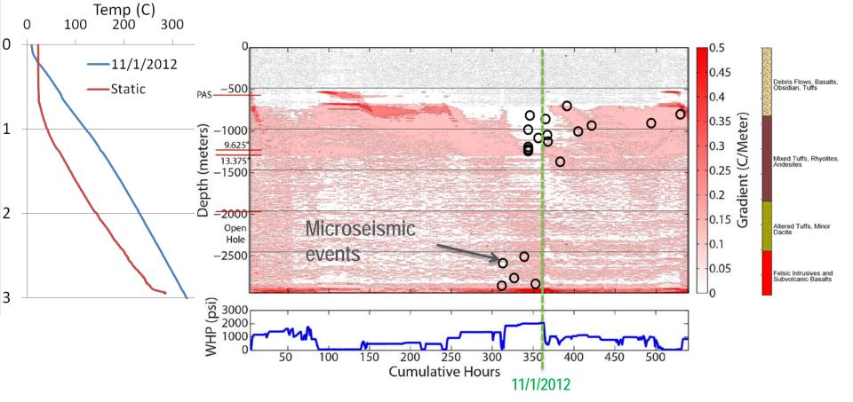
Although seismicity occurred above depth of 1500 m bgs, temperature profiles and gradients over 550 hour period indicate majority of fluid exited below 2500 m depth.
