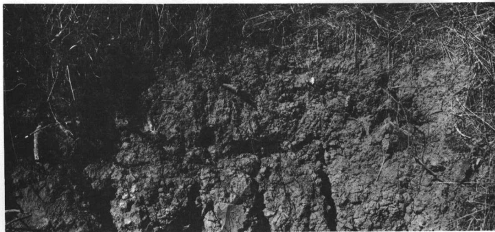
Figure 5.—Profile of Hazelair silt loam, 3 to 12 percent slopes. Wide vertical cracks in the subsoil are caused by a high shrink-swell clay.
