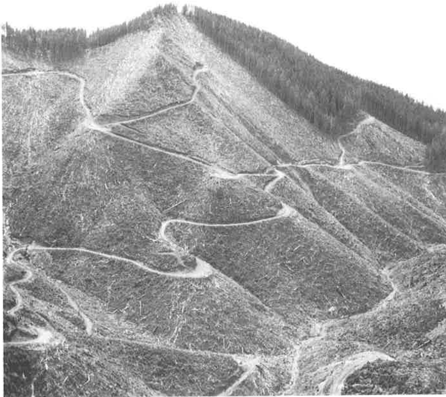
Extensive clear-cuts and roadbuilding on Neahkahnie Mountain adjacent to Oswald West State Park (summit trees) expose the steep slopes to landslides (Photo courtesy Oregon Department of Transportation)
