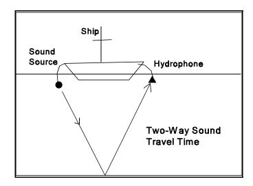
Example Problem: If the source-hydrophone travel time is 2 sec, what is the depth of the sea floor directly below a ship?
