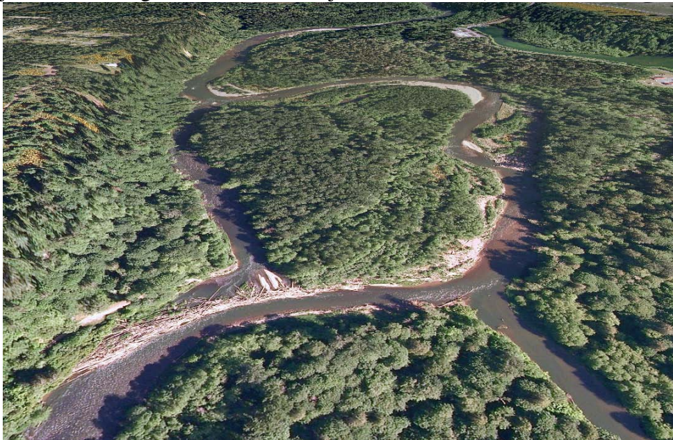
Figure 11. Oblique aerial view of a large meander-bend log jam on the Nisqually River. The jam serves to regulate flow into a major side-channel (Thurston and Pierce Counties, WA).
