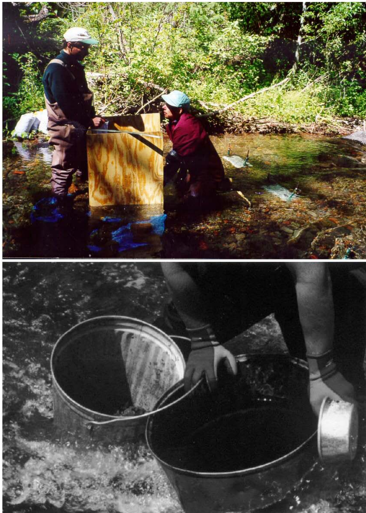
Figure 1. Two types of shields for isolating a portion of the streambed from water flow in order to collect bulk sediment samples. Top: three-sided plywood shield (photo: Paul Bakke). Bottom: barrel sampler (photo: Kristin Bunte).
