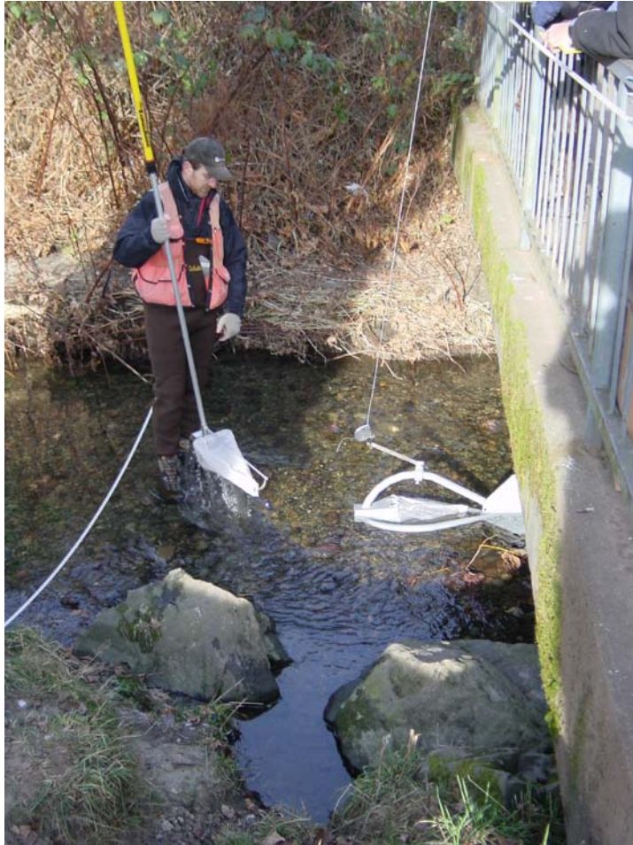
Figure 3. Helley-Smith bedload samplers. Handheld model is on left. Model on right is for use with reel and cable equipment.
