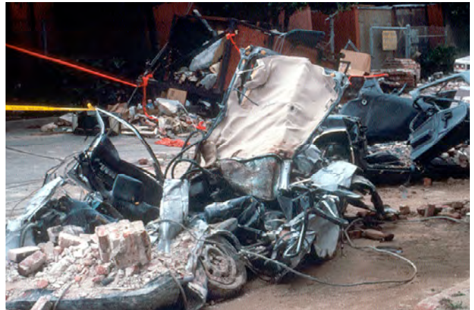
Ground response at different locations means there can be dramatically different levels of damage in the same quake. This car, crushed in the 1989 Loma Prieta, California earthquake, was in an area where there was a great deal of building failure. Falling bricks or parapets can cause injuries and damage on the streets and sidewalks below. Photo: C. E. Meyer, USGS
