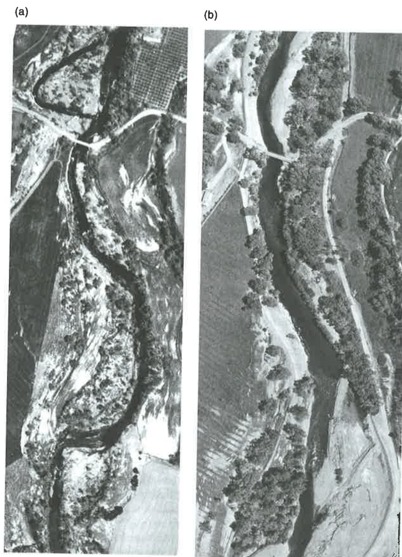
Figure 21.5 Details from aerial photographs of Deer Creek near Leininger bridge in 1939 and 1997. Flow is from top to bottom, length of river shown is about 1100 m. (a) The 1939 channel was more complex, sinuous, and with more frequent bed variations, gravel bars, and undercut banks with adjacent riparian vegetation. (b) The 1997 channel is less sinuous, wider, and less complex, reflecting the effects of the 1949 flood control project, and subsequent maintenance. Also visible in the 1997 photo detail is the levee breach along the left (south) bank
