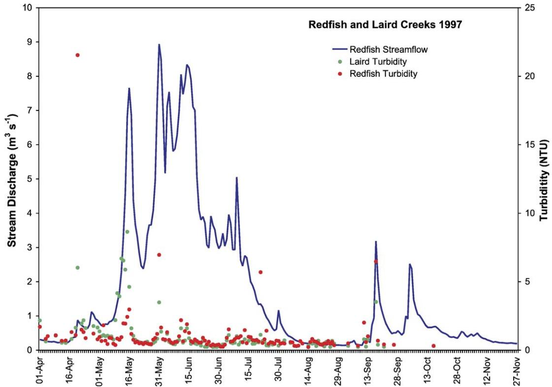
Fig. 6. Example of a hydrograph of mean daily discharge for Redfish Creek for one season, and turbidity samples for Redfish and Laird Creeks.
