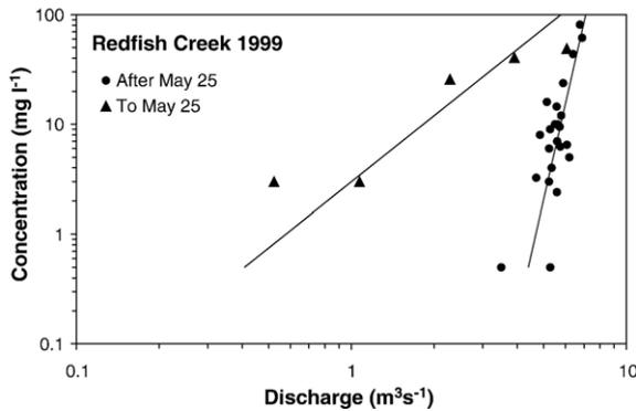
Fig. 5. Example of a discharge–concentration curve, used to estimate suspended sediment concentration for days when no water sample was taken. Left cluster of points (triangles) is early season samples (to May 25 in this example); right cluster (dots) is the remainder of the spring runoff period. The lines are fit by eye.
