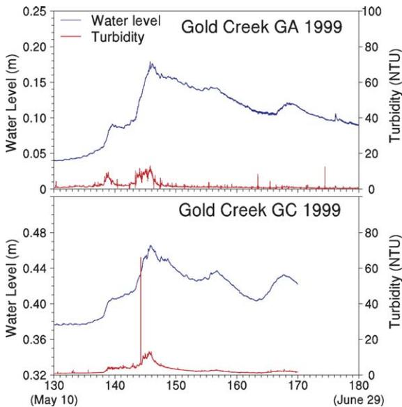
Fig. 8. Water level and turbidity for two tributaries of Gold Creek. Time period and measurements are the same as for Fig. 7. Water level for GC is measured to an arbitrary datum. Top: GA, with recent logging and road construction. Bottom: GC, the undeveloped tributary.
