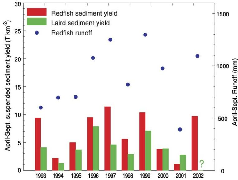
Fig. 10. April–September suspended sediment yields for Redfish and Laird Creeks, and runoff for Redfish Creek, for the 10-year period of record. The 2002 yield for Laird Creek is missing, as bedload movement interfered with the automatic pump sampler.
