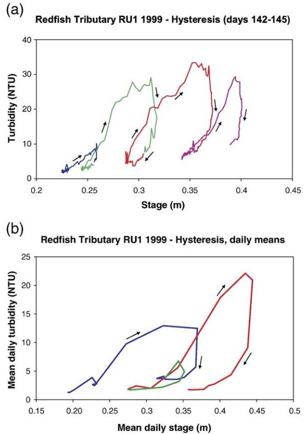
Fig. 9. Graphs showing hysteresis of turbidity. The data are from the turbidity and water level record shown in Fig. 7. (a) Four days of record (days 142–145) during a peak snowmelt period; data points are every 15 min. (b) Daily mean turbidity and water level for a 4-week period which includes most of the seasonal snowmelt runoff.
