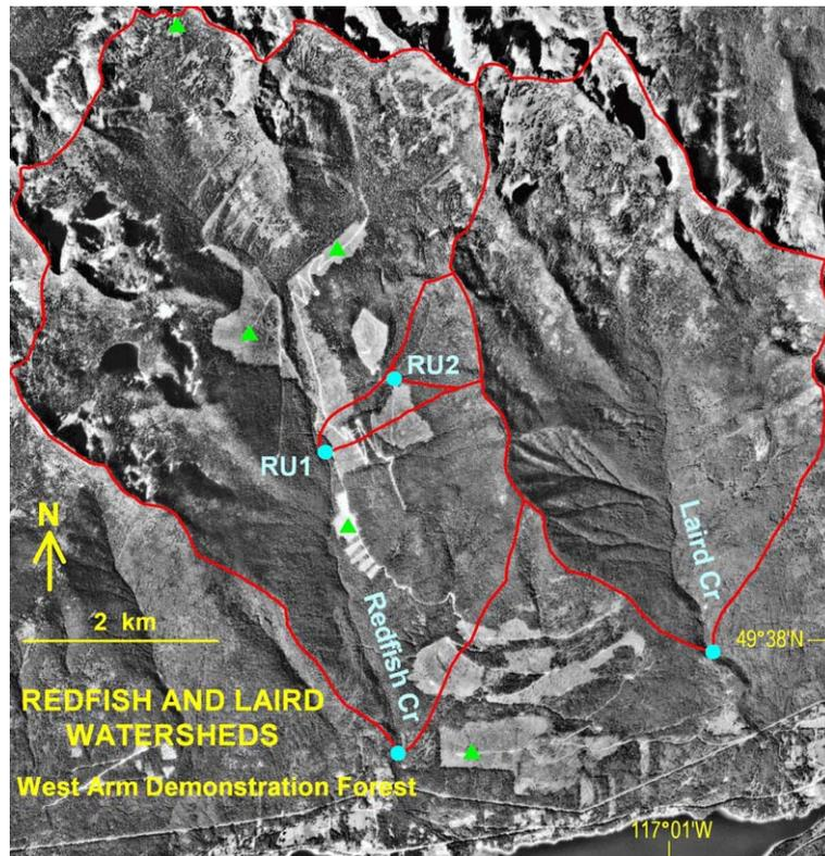
Fig. 2. Map of Redfish Creek and Laird Creek watersheds, based on an orthophoto. Round dots are streamflow and sediment monitoring stations. RU1 and RU2 are the lower and upper stations, respectively, in the Redfish Upper tributary. Triangles are climate stations.
