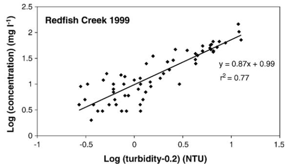
Fig. 4. Example of a turbidity–concentration curve. Horizontal axis ( $x$ ) is log of turbidity minus 0.2 NTU; this is used because turbidity converges on a value of 0.2 NTU when suspended sediment concentration is zero. Vertical axis ( $y$ ) is log of suspended sediment concentration.
