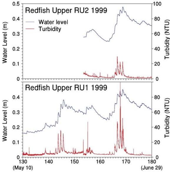
Fig. 7. Water level and turbidity for two sites on the Redfish Upper tributary for the snowmelt season of 1999. Horizontal axis gives the day of the year. The turbidity graph is output from the OBS meter, uncorrected for false signals or drift of the instrument zero. Water level is measured to the lowest point of the weir edge. Data are recorded at 15-min intervals. Top: upper site (RU2). Bottom: lower site (RU1).
