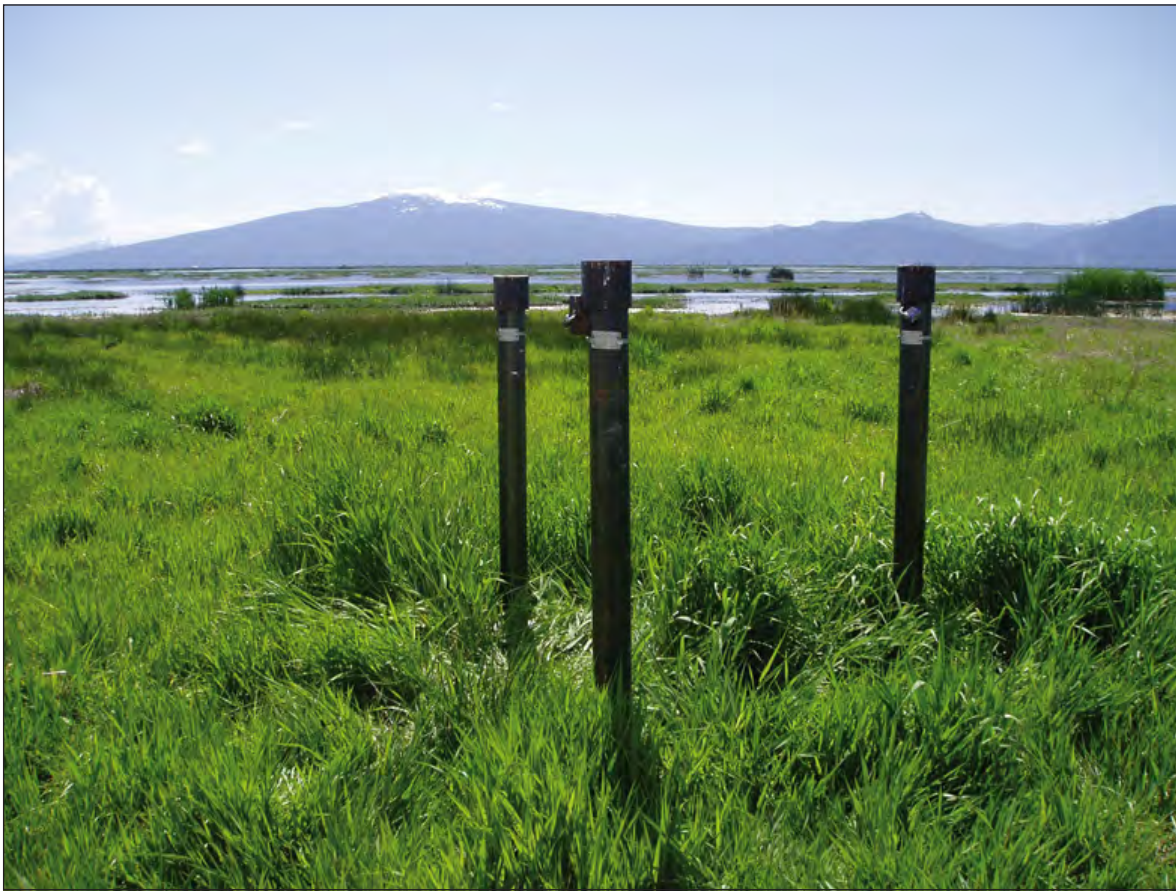
Ground-water piezometer nest in the South Unit of the Wood River Wetland (looking west southwest). Photograph taken by Kurt Carpenter, U.S. Geological Survey, June 2004.
