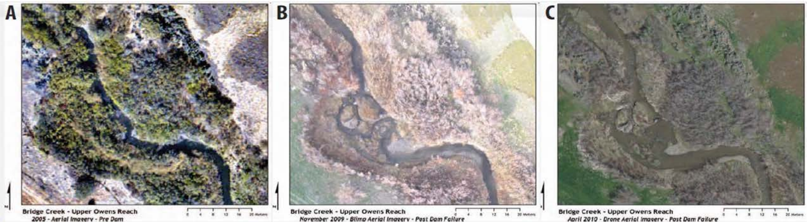
Figure 10: Progression of reach at upper Owens through a period without a dam (A; 2005), with an active, partially breached dam (B; Nov 2009), to an abandon, partially breached dam (C; April 2010).
