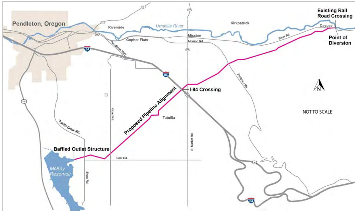
Figure 3. Schematic of McKay Reservoir Enlargement gravity diversion alternative.
