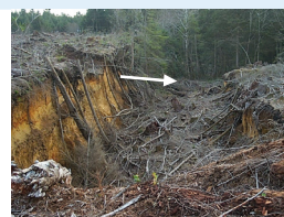
translational slide (most slides are combinations of translational and rotational movement)
