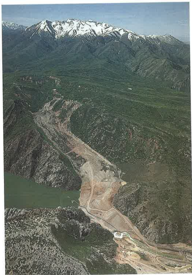
▲ FIGURE 6.20 Thistle landslide, Utah. This landslide, which occurred in 1983, involved the reactivation of an older slide. The landslide blocked the canyon, creating a natural dam, flooding the community of Thistle as well as the Denver-Rio Grande Railroad and a major U.S. highway. (Michael Collier)
