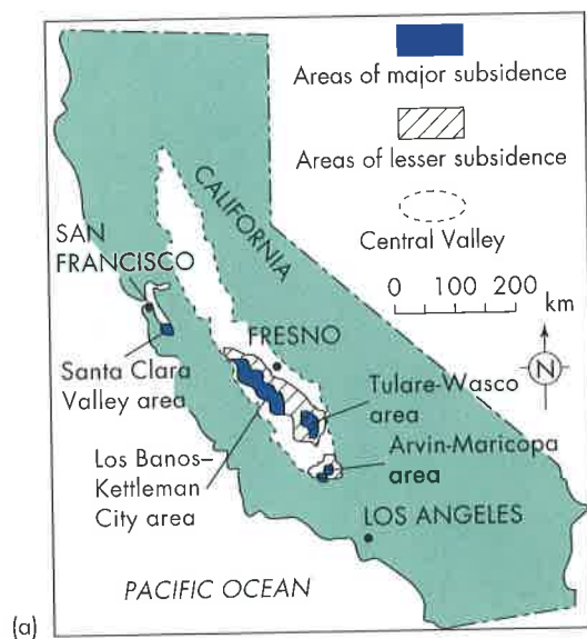
▲ FIGURE 6.22 (a) Principal areas of land subsidence in California resulting from groundwater withdrawal. (After W. B. Bull, 1973. Geological Society of America Bulletin 84. Reprinted by permission.) (b) Photograph illustrating the amount of subsidence in the San Joaquin Valley, California. Marks on telephone pole are positions of the ground surface in recent decades. The photo shows approximately 8 m of subsidence. (Courtesy of Ray Kenny)
