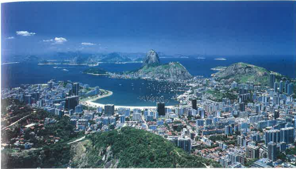
◀ FIGURE 6.16 Panoramic view of Rio de Janeiro, Brazil, showing the steep (sugarloaf) hills. Combination of steep slopes, fractured rock, shallow soils, and intense precipitation contribute to the landslide problem, as do human activities such as urbanization, logging, and agriculture. Virtually all of the bare rock slopes were at one time vegetated, and that vegetation has been removed by landsliding and other erosional processes. (Tony Stone Images)
