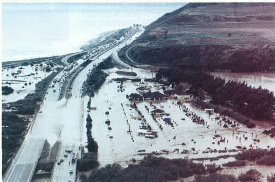
► FIGURE 5.E Flooding of the Ventura Beach RV Resort in February 1992. The RV park was built directly across a historically active distributary channel of the Ventura River delta. The recurrence interval of this flood is approximately 22 years. A similar flood occurred again in 1995. Notice that U.S. Highway 101 along the Pacific Coast is completely closed by the flood event. (Mark J. Terrell/AP/Wide World Photos)
