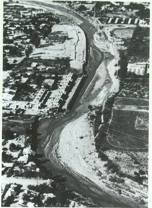
► FIGURE 5.D Tucson flood damage on the Rillito in 1983. Flow is from bottom to top in the photograph. Note damage to townhouses (center) due to lateral migration of the upstream meander bend that eroded behind and through bank protection (soil cement) emplaced to protect the houses. (Edward A. Keller)
