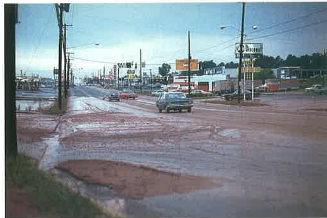
▲ FIGURE 3.9 Soil erosion has caused unwanted red sediment at this site in Charlotte, North Carolina. (Edward A. Keller)
