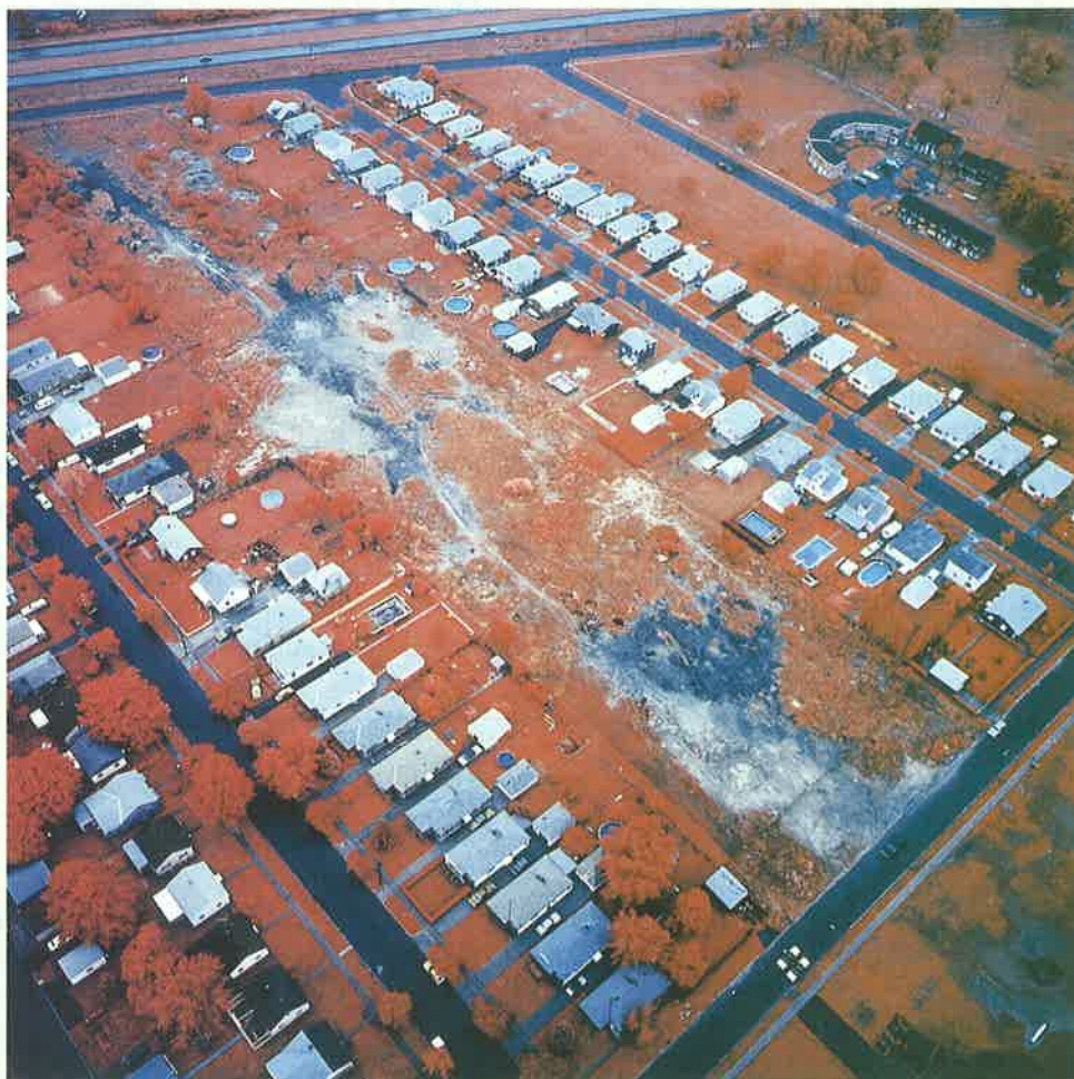
▲ FIGURE 12.B This is an aerial infrared photograph of the Love Canal area in New York. Healthy vegetation is bright red. This portion of Love Canal runs from the upper left corner to the lower right. It appears as a scar on the landscape. Buried chemical waste seeped to the surface to cause numerous environmental problems and concern here. The site became a household name for toxic waste. (New York State Department of Environmental Conservation)
