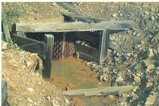
▲ FIGURE 11.C Water seeping from this Colorado mine is an example of acid mine drainage. The water is also contaminated by heavy metals. (Tim Haske/Profiles West/Index Stock Imagery, Inc.)
