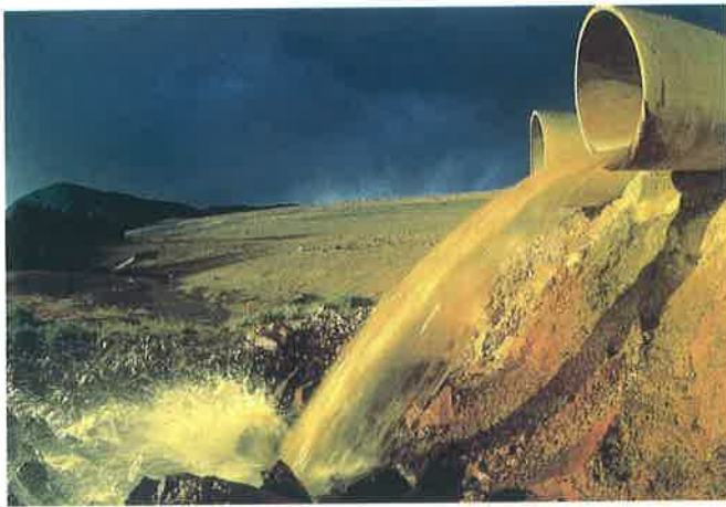
▲ FIGURE 11.5 Pipe discharging partially treated effluent from the Climax Molybdenum Mine in Colorado. (Jim Richardson/Richardson Photography)
