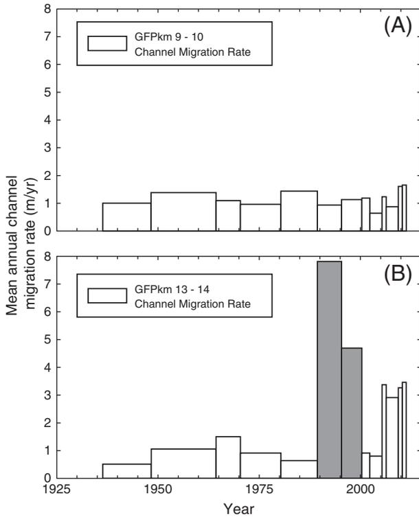
**Fig. 8.** Mean annual channel migration rate (A) between GFPkm 9 and 10 and (B) GFPkm 13 and 14. Migration rates greater than the total error from orthorectification and digitization are shaded gray.
