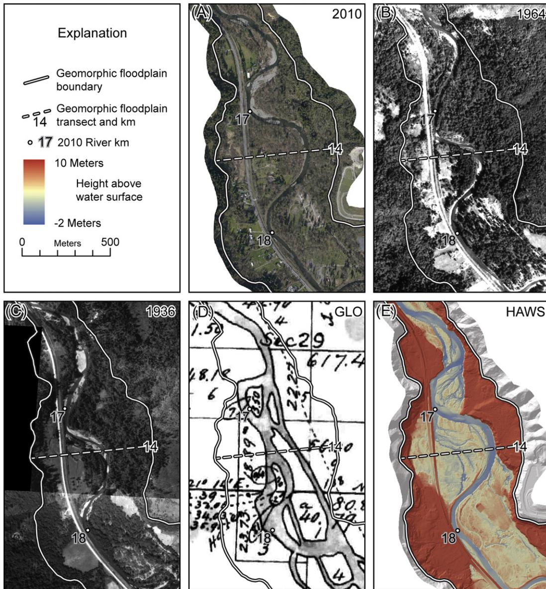
**Fig. 10.** Progression of planform geomorphic features in the vicinity of GFPkm 14: (A) 2010 orthoimagery, (B) 1964 orthoimagery, (C) 1936 orthoimagery, (D) 1865–1880 General Land Office (GLO) survey, and (E) height above water surface (HAWS).
