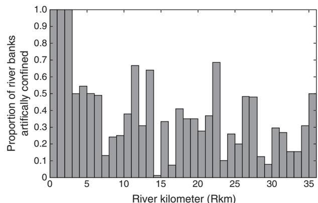
**Fig. 4.** Proportion of river banks artificially confined by revetments or other bank stabilization structures in 2010.
