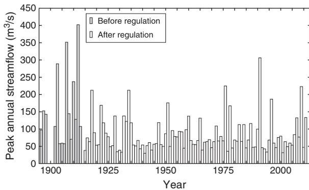
**Fig. 2.** Annual peak streamflow of the Cedar River near Landsburg (U.S. Geological Survey streamflow-gaging station 12117500) for water years 1896–1898, 1902–1913, and 1915–2011. Peak annual streamflows before regulation in 1914 are shaded.
