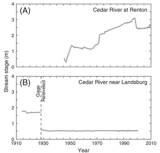
**Fig. 9.** Temporal variations in stream stage for the median streamflow at USGS streamflow gaging stations at (A) Renton (12119000) and near (B) Landsburg (12117500) on the Cedar River.
