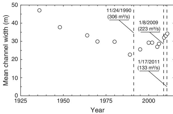
**Fig. 7.** Mean channel width for the Cedar River downstream of the Landsburg diversion dam measured from 13 orthoimagery sets between 1936 and 2011. The time of notable peak streamflows measured near Landsburg at USGS streamflow gaging station 12117500 is shown by vertical dashed lines.
