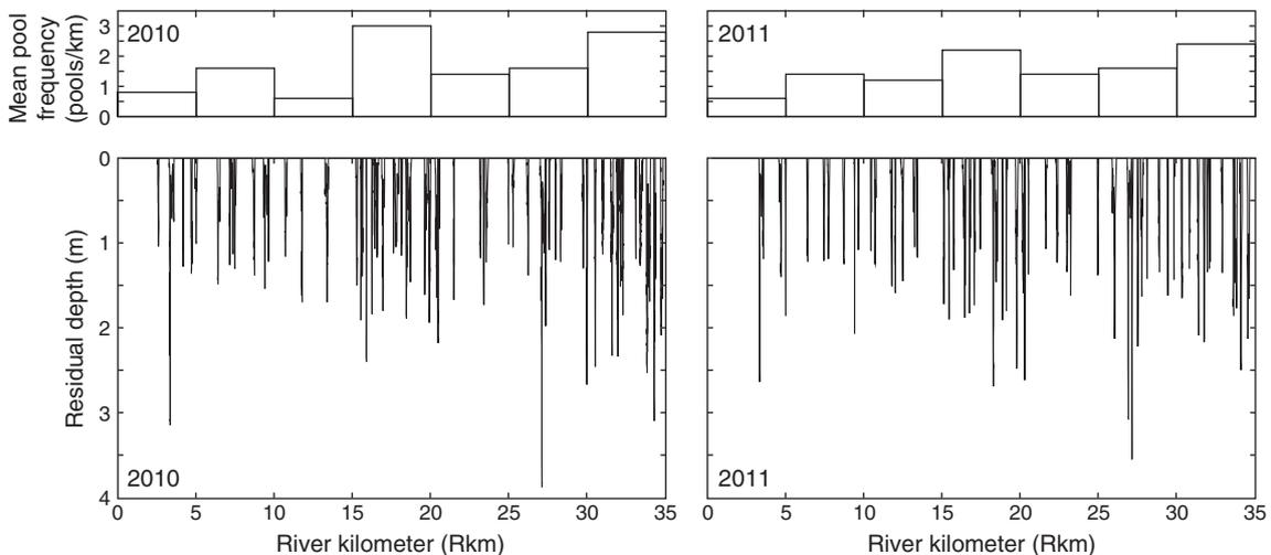
**Fig. 6.** Residual pool depth and frequency between Rkm 0 and 35 surveyed in April 2010 and July 2011.
