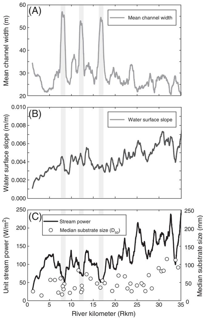
**Fig. 5.** Longitudinal variation in active-channel width, water-surface slope, stream power, and median substrate size ( $D_{50}$ ) of the Cedar River between Rkm 0 and 35. Gray areas indicate longitudinal extent of unconfined reaches in between Rkm 7.5–8.5, Rkm 11.5–12.5, and Rkm 16.0–17.0.
