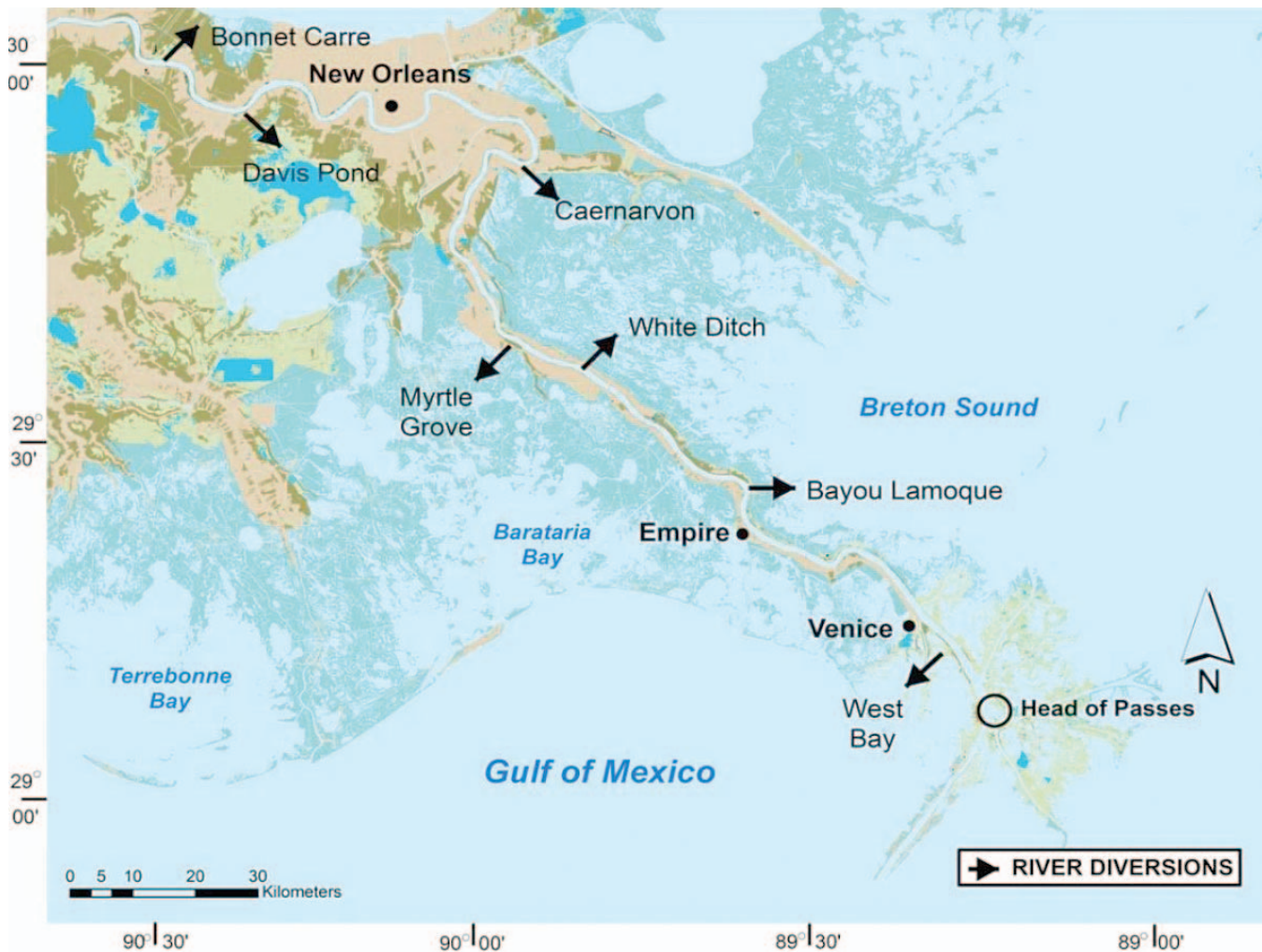
Figure 2. Existing and planned diversions along the lower course of the Mississippi River. Land-building in the birdsfoot delta (SE of Venice) is shown in the four subdeltas in Figure 3. See CPRA (2012) for summary of planned diversions.
