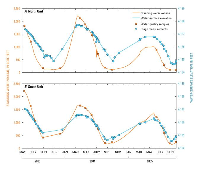
**Figure 5.** Daily water-surface elevations and standing volumes in the (*A*) North Unit and (*B*) South Unit of the Wood River Wetland, upper Klamath River basin, Oregon, 2003–05. (Dates of stage measurements and collection of water-quality samples for each unit are indicated.)
