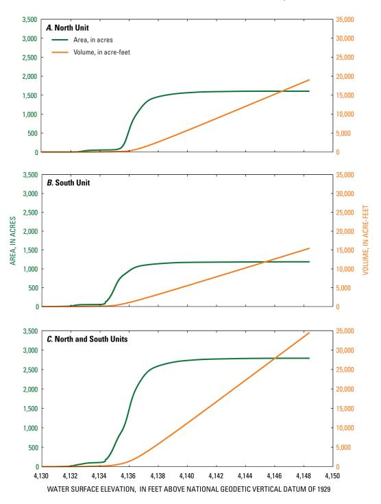
**Figure 4.** Stage, volume, and area relations for the (*A*) North Unit, (*B*) South Unit, and (*C*) North and South Units of the Wood River Wetland, Oregon.
