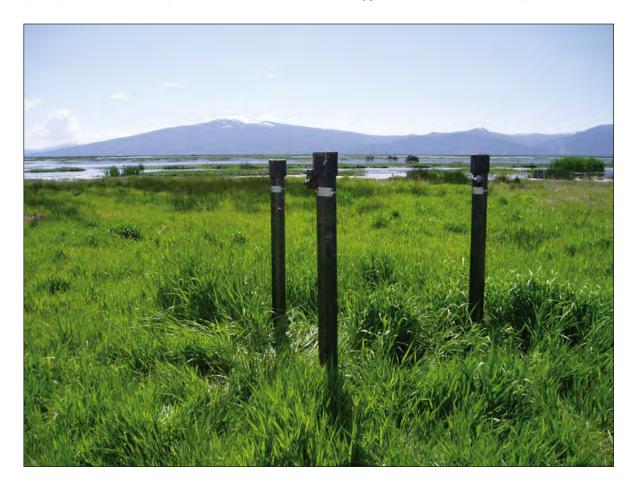
Ground-water piezometer nest in the South Unit of the Wood River Wetland (looking west southwest). Photograph taken by Kurt Carpenter, U.S. Geological Survey, June 2004.
