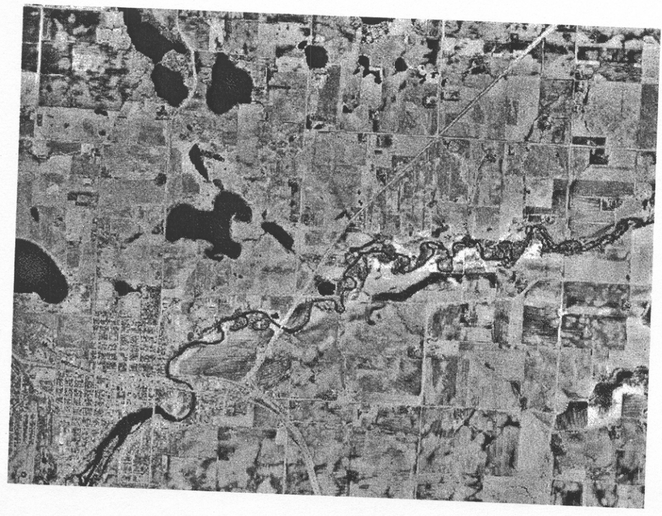
Figure 4.5 This example of aerial photography available from the U.S. Geological Survey's EROS Data Center is the type of image that provides geomorphologic information, including channel width, sinuosity, and pattern, as well as floodplain dimensions. The image is of terrain in southern Minnesota. Source: EROS Data Center ( http://edcwww.cr.usgs.gov ).
