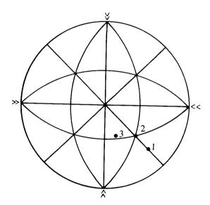
112. On the stereogram above, the great circles represent planes inclined 45 degrees to the three axes (east-west, north-south, and vertical), and all three points on the stereogram (1, 2, 3) have Miller indices of 111. Which of the following correctly identifies the crystal system each point represents?
