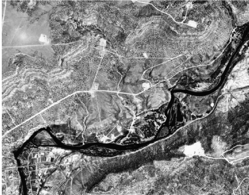
Fig. 3. Channel shrinkage from Navajo Dam and water diversions have converted the San Juan River, N.M., from a braided planform to a single thread channel. U.S. Geological Survey aerial photograph, EROS Data Center.
