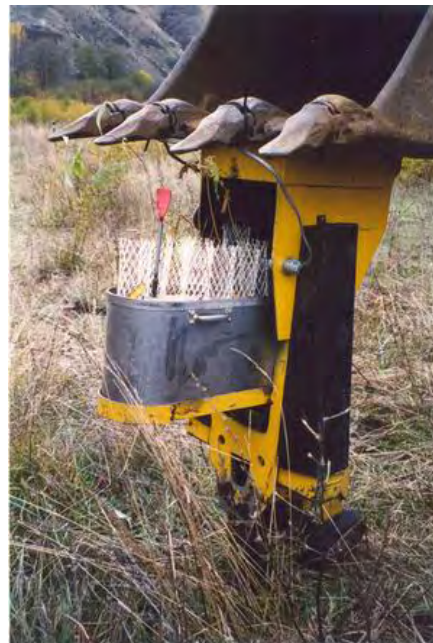
Riparian Restoration and Management Figure 5: Expandable stinger variation capable of planting 3”-diameter rooted-plant plugs into unarmored streambanks at a rate of up to three hundred per hour.
