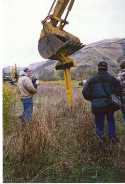
Riparian Restoration and Management Figure 4: Expandable stinger for live stakes and 3” plugs. It has been used to plant 30 to 250 cuttings per hour, depending upon site conditions.
