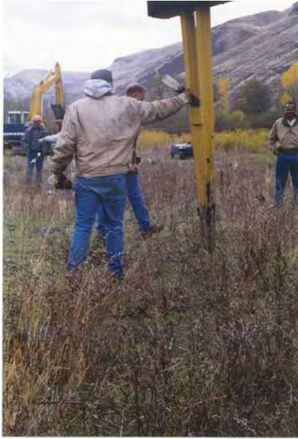
Riparian Restoration and Management Figure 4: Expandable stinger for live stakes and 3” plugs. It has been used to plant 30 to 250 cuttings per hour, depending upon site conditions.
