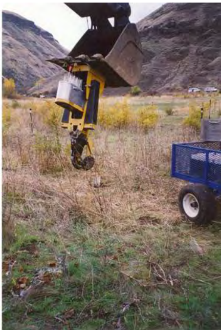
Riparian Restoration and Management Figure 5: Expandable stinger variation capable of planting 3”-diameter rooted-plant plugs into unarmored streambanks at a rate of up to three hundred per hour.
