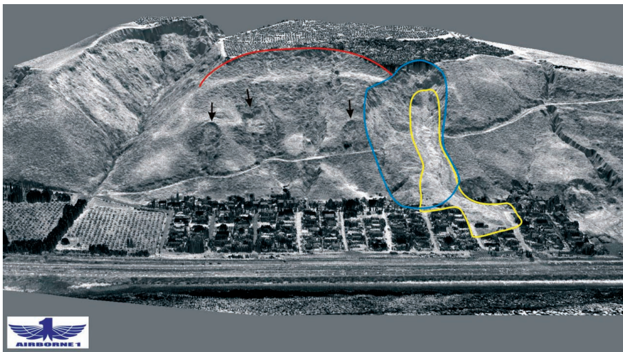
Figure B7. An oblique LiDAR image of La Conchita, California, USA, landslide, taken in 2005. Outline of 1995 (blue) and 2005 (yellow) landslides are shown; arrows show examples of other landslides in the area; red line outlines main scarp of an ancient landslide that involved the entire bluff. (Photograph by Airborne 1, El Segundo, California, USA, and Randy Jibson, U.S. Geological Survey.)
