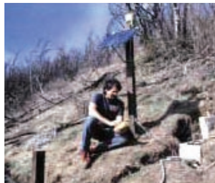
Figure B9. Testing a solar-powered radiotelemetry system for remote transmission of real-time landslide data. (Photograph by Mark Reid, U.S. Geological Survey.)
