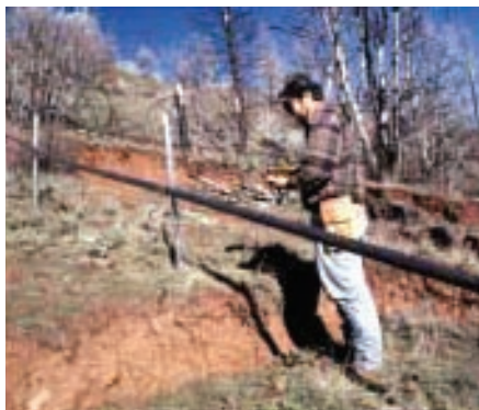
Figure B8. Measuring landslide movement using an extensometer, an instrument that can detect movement of the ground surface between stable ground and sliding ground. (Photograph by Richard LaHusen, U.S. Geological Survey.)
