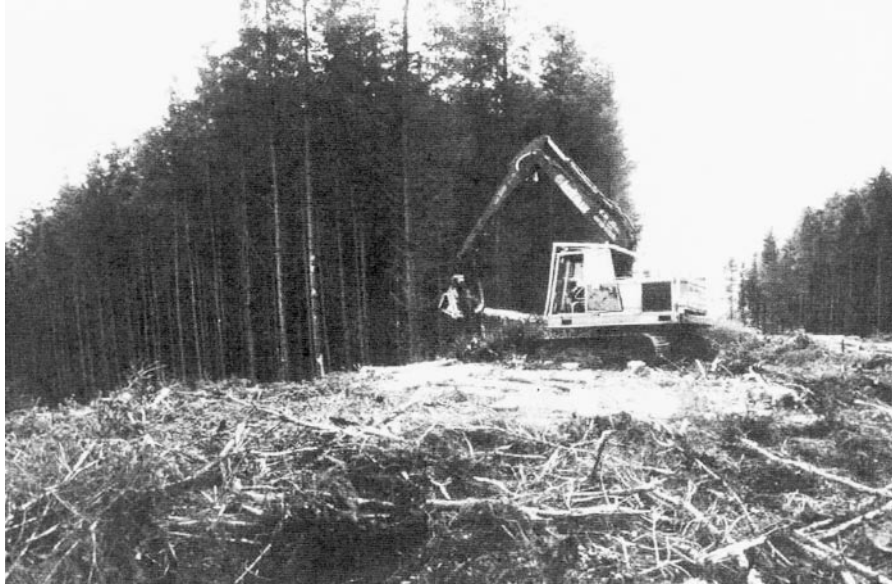
Figure 2. One machine timber harvester processing felled tree, Plynlimon.
