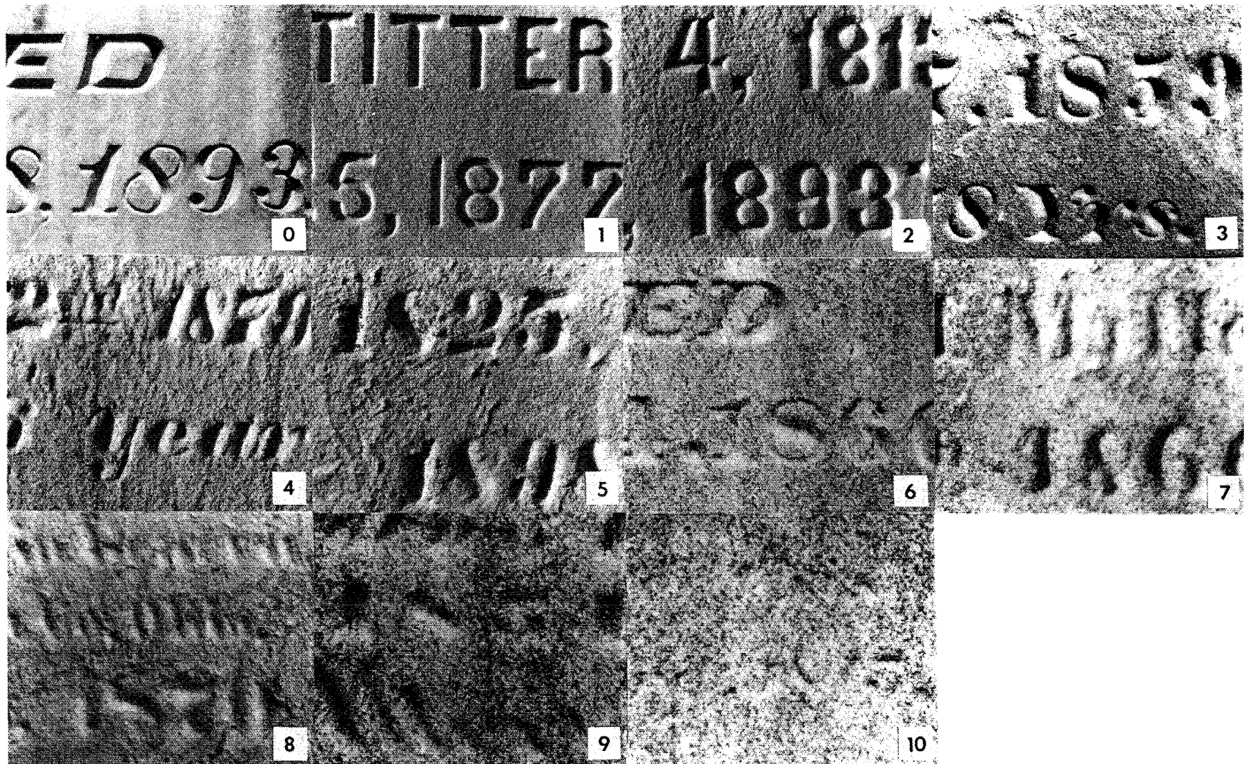
Fig. 1. Photographic comparison scale of inscription legibility states (0-10) on Vermont marble tombstones at various North American locations. No photo is available for state 11 (no visible trace remaining of original inscription).
