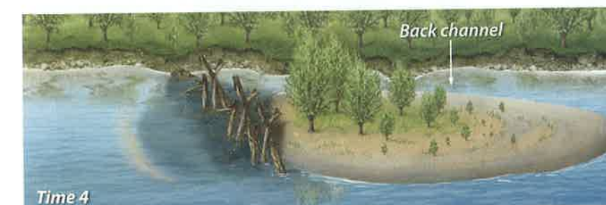
FIGURE 6.11 Effects of Large Woody Debris. Large woody debris in channels changes the distribution of water flow and velocity.
