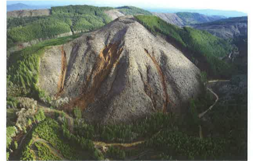
FIGURE DD5.5 Debris flows off a steep, clear-cut slope, Stillman Creek, Washington. The timber company's application to the State Department of Natural Resources before harvest reported that the site had been inspected and was found to have no potentially unstable slopes. [Photograph by S. Ringman, from Seattle Times .]
