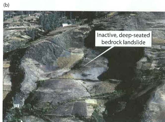
PHOTOGRAPH 5.10 Active and Inactive Landslides. Recently active and older inactive landslides can easily be distinguished. (a) An active shallow planar landslide, near Florence, Oregon, has recently disrupted a steep forested slope. The slide was likely triggered by wave erosion at the toe of the slide. (b) Inactive, deep-seated bedrock landslide with well-defined scarp in the Bolivian Andes. Landslide is currently stable enough that it is crossed by roads and covered by agricultural fields.
