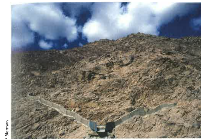
PHOTOGRAPH 5.19 Bedrock Hillslope. Bare rock hillslope (weathering limited) at the Nahal Yael experimental watershed in the Negev Desert, Israel. Here, runoff from the bare granite hillslope is funneled into a weir so that it can be measured.
