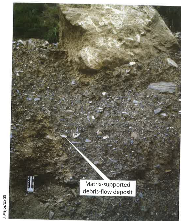
PHOTOGRAPH 5.14 Debris-Flow Deposit. Bouldery debris flow deposit in the Jiangjia River Valley of China, showing the matrix-supported nature of material deposited by the flow. The large boulder at the top of the photo was carried by the flow.
