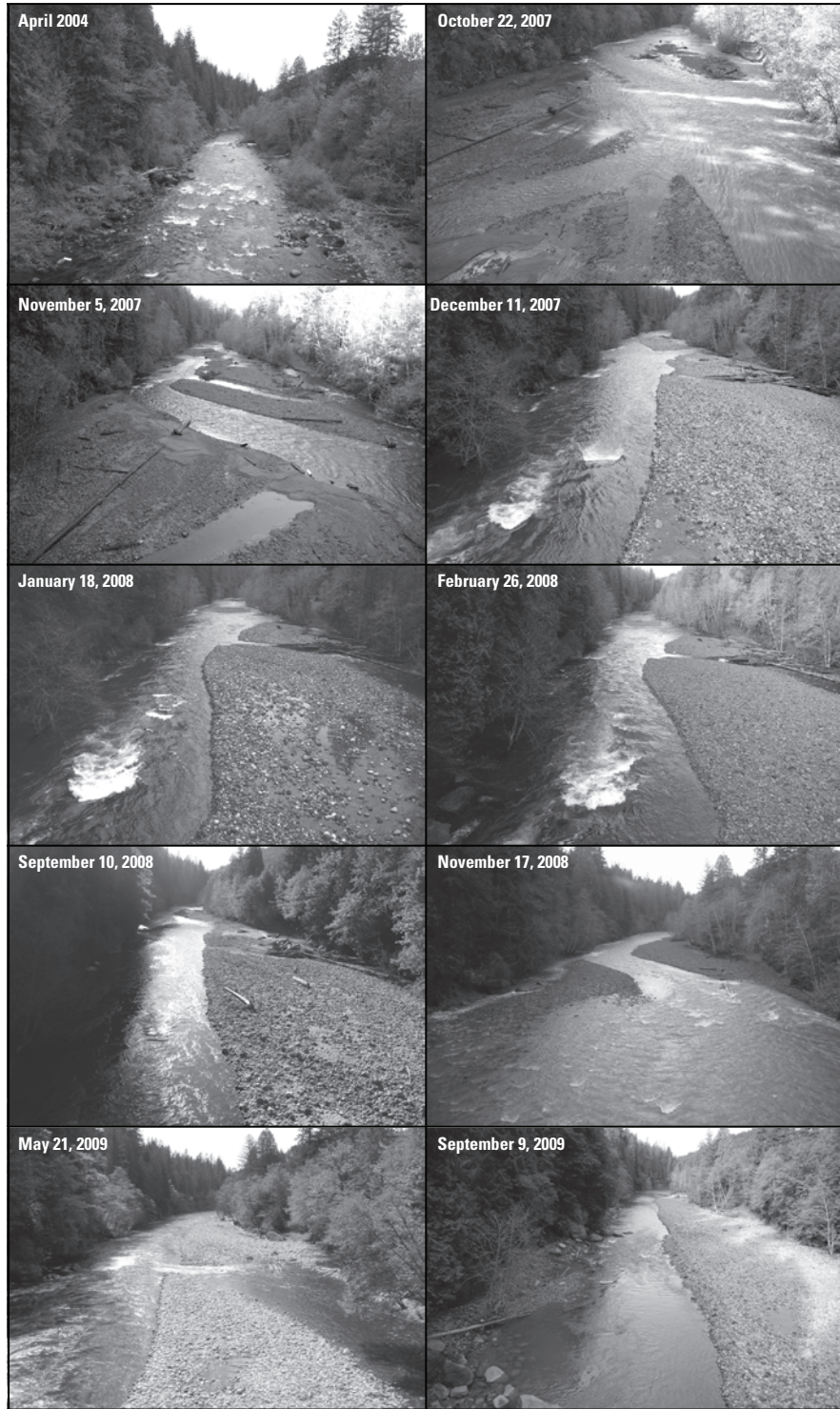
Figure 22. Time series of photographs of Sandy River from pedestrian bridge at Marmot Dam site. View is downstream; field of view is ~40 meters wide. Following the October 19, 2007, breaching, the channel rapidly aggraded and transitioned from the single-thread boulder-cobble channel shown in the April 2004 photograph to the multithread sand-and-gravel channel shown by the October 22 and November 5, 2007 photographs. By December 2007, the channel reverted to a single thread flanked by coarse gravel bars, although these bars show evidence of being remobilized by the higher flows that occurred during the second year after breaching, such as that in November 2008.
