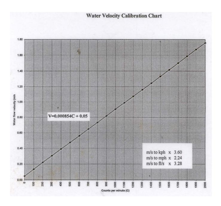
To convert flow velocity from "revolutions per minute" to m/sec; Multiply the count x 0.000854 and add 0.05
