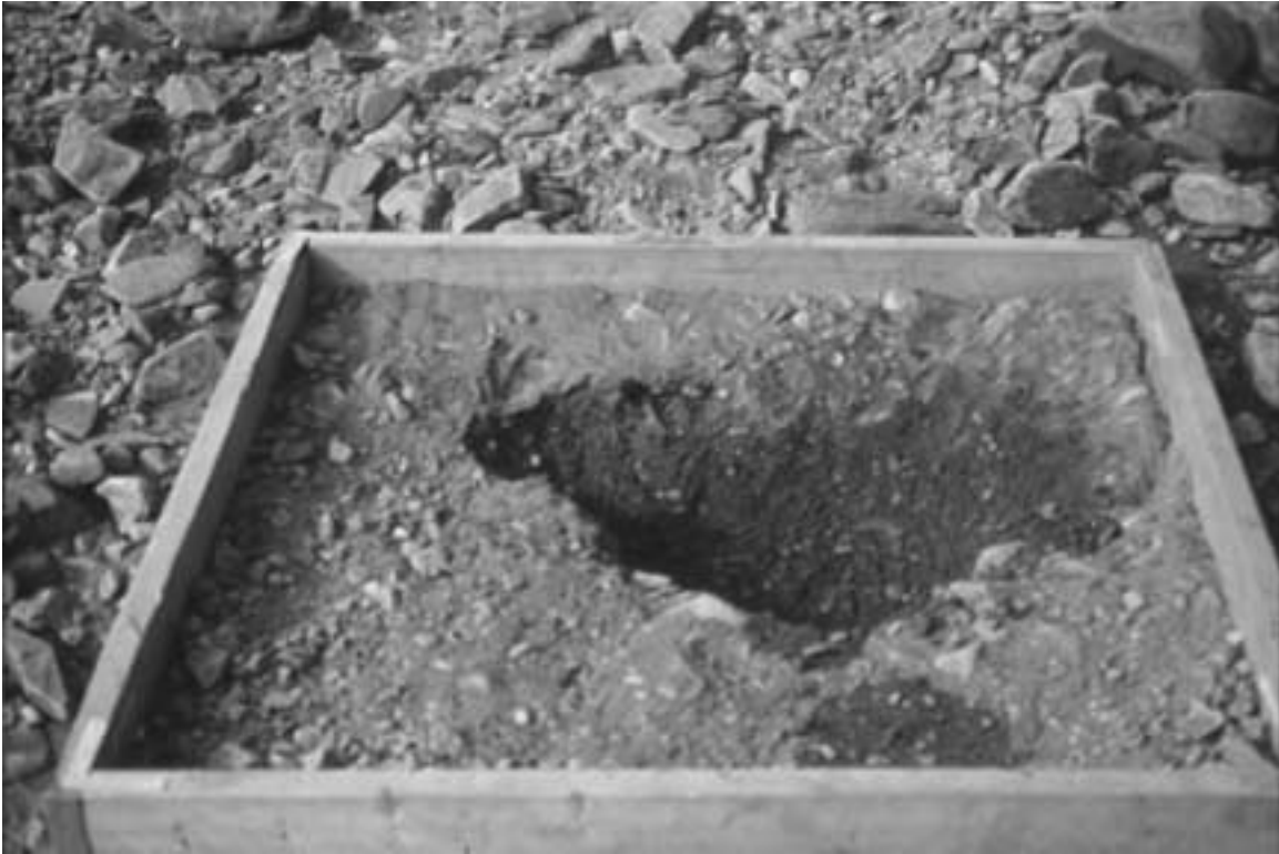
Fig. 2.31: Frame for measuring in situ subsurface sediment bulk density (Photo courtesy of R. Milhous).
