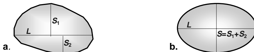
Fig. 4.13: Axes L , S_1 and S_2 fitted by computer into the outlined and digitized particle shape (a); Computer-fitted ellipsoidal reference particle shape for computation of particle volume (b). (Redrawn from Ibbeken and Schleyer (1986), by permission of John Wiley and Sons, Ltd.).
