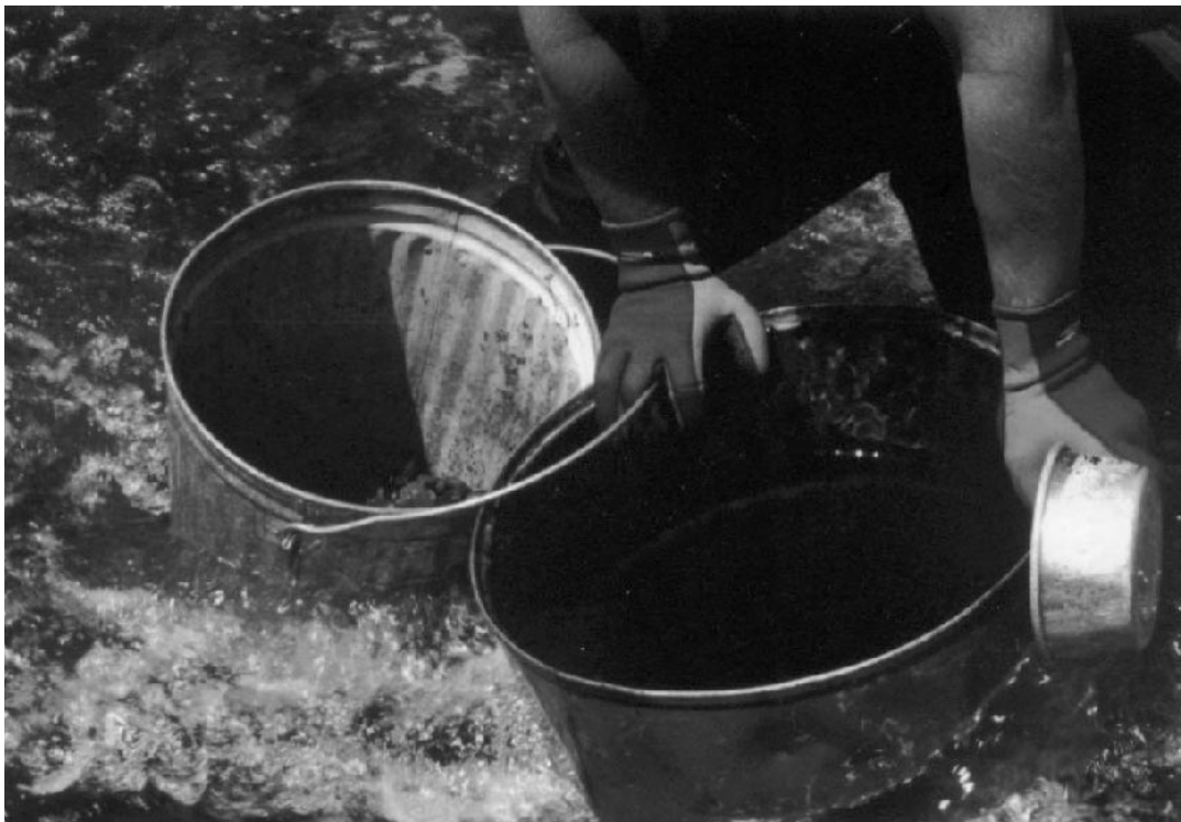
Fig. 4.26: Taking a barrel sample, South Fork Cache la Poudre Creek, Colorado. (Photograph by K. Bunte).
