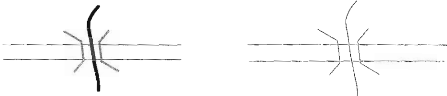
The Image Thinning command reduces lines in an image to one pixel wide.
