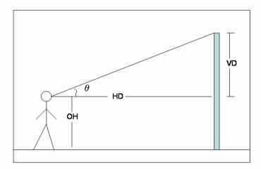
OH = ocular height, VD = vertical distance from eyes to top of object, HD = horizontal distance from eyes to object,  $\theta$  = angle of inclination between eyes and top of pole:
