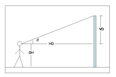
OH = ocular height of persons eyes from ground surface,  $VD = vertical distance from eyes to top of object, HD = horizontal distance from eyes to object, <math>\theta = angle of inclination between eyes and top of pole using a clinometer:$
