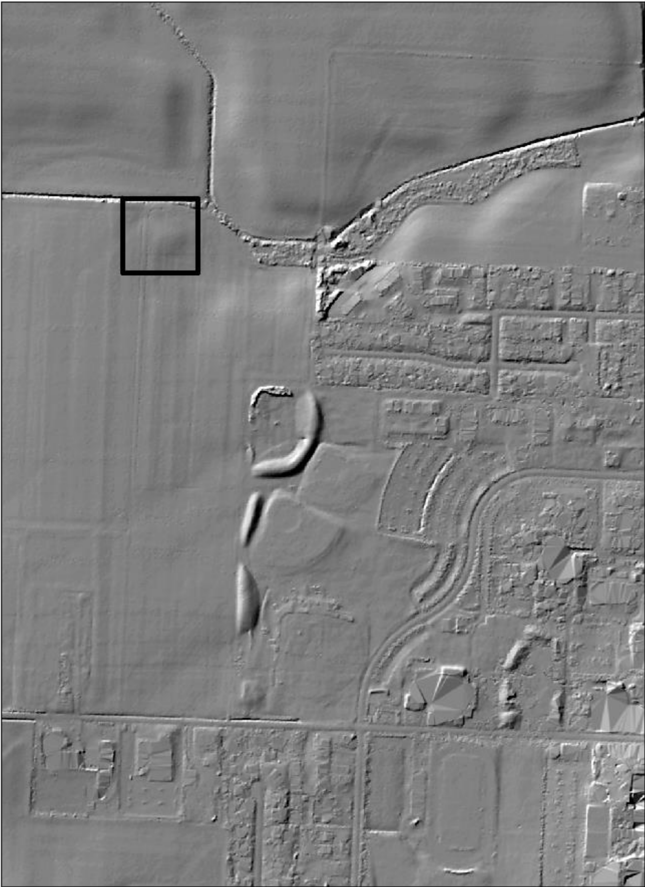
LiDAR-Based Hillshade Model of the WOU Field Site (1-m resolution)
