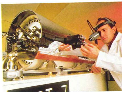
▲ This atomic clock, which keeps time on the basis of radiation from cesium atoms, is accurate to about three millionths of a second per year. (How long would it take for it to gain or lose an hour?)
