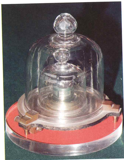
▲ The standard kilogram, a cylinder of platinum and iridium 0.039 m in height and diameter, is kept under carefully controlled conditions in Sèvres, France. Exact replicas are maintained in other laboratories around the world.
