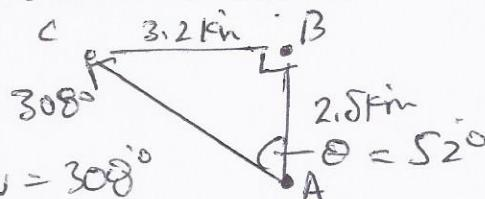
$$\text{Bearing } AC = \\ 360 - 52^\circ = \\ 308^\circ$$
