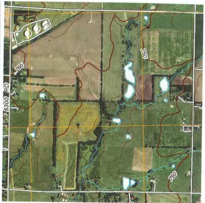
B. Orthoimage base with all other data layers: contour lines, UTM grid lines (WGS84, Zone 15S), geographic names and boundaries, hydrography, and transportation features.
