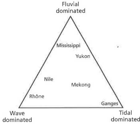
Fig. 6.9 Classification of delta types using a triangular diagram.
