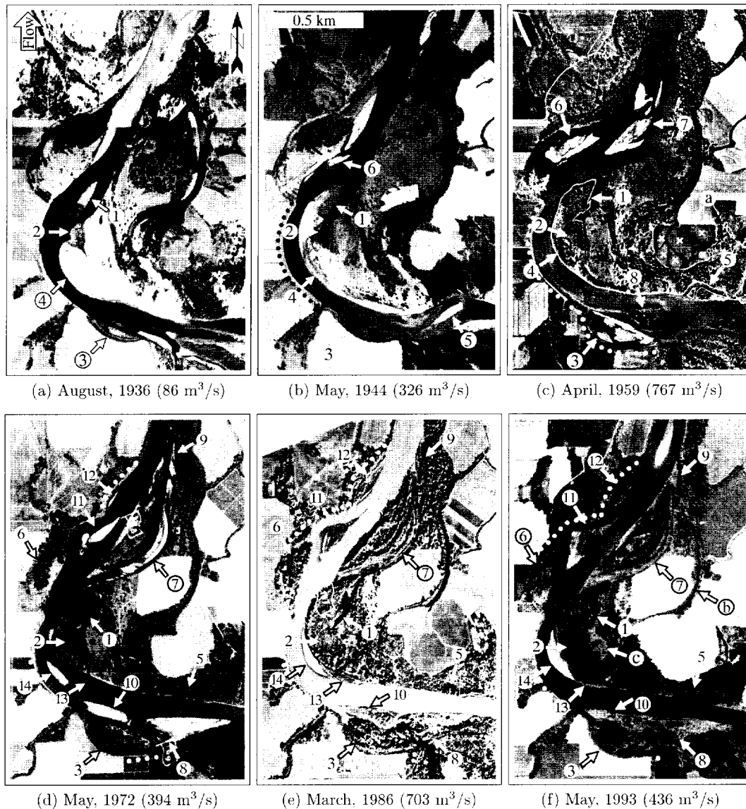
Figure 4. Historical series at river km 269, with calendar year and flow at the Albany gage given below each photograph. Scale bar is shown in the 1944 frame. Dotted lines, black or white, show location of shoreline revetments.
