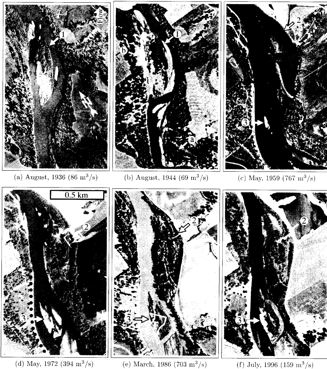
Figure 5. Historical series at river km 216, with calendar year and flow at the Albany gage given below each photograph. Scale bar is shown in the 1972 frame. Dotted lines, black or white, show location of shoreline revetments.
