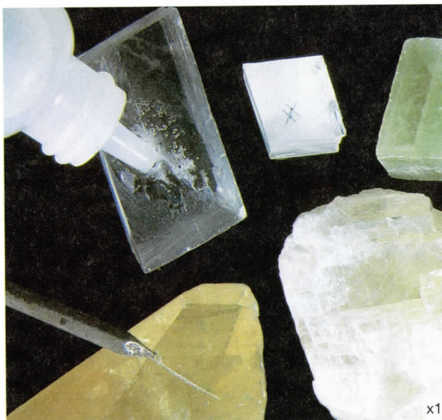
FIGURE 3.16 Acid test. Place a drop of weak hydrochloric acid (HCl) on the sample. If it effervesces (reacts, bubbles), then it is a carbonate ( \text{CO}_3 -containing) mineral. Please wipe the sample dry with a paper towel after doing this test! Note that the mineral in this example occurs in several different colors and can be scratched by a wire (iron) nail. The yellow sample is a crystal of this mineral, but the other samples are broken pieces of crystals that reveal the mineral's characteristic cleavage angles.
