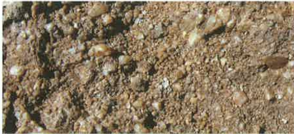
C. Sandstone cemented with yellow to brown limonite.
