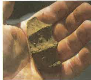
FIGURE 6.4 Compaction of mud to form mudstone. The more the mud (silt and clay sized grains of detrital sediment) is compacted, the harder (more lithified) it will become. Deeply buried mud is also lithified by heat as it is compacted, like baking clay pots in a kiln.
