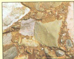
Breccia: made mostly of angular gravel (usually rock fragments)
