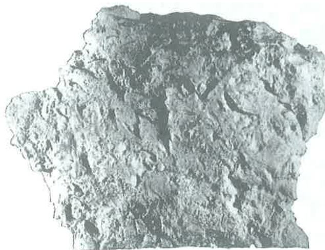
FIGURE 6.3 Portland limestone (Upper Jurassic) showing biomoldic porosity due to solution of shells. Portland Island, Dorset, United Kingdom.
