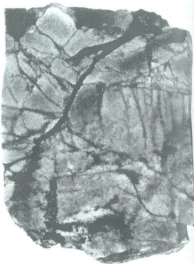
FIGURE 6.5 Fractured core of Gargaf Group sandstone (Cambro-Ordovician). Sirte basin, Libya.
