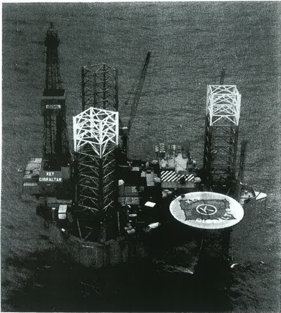
FIGURE 3.8 Jack-up drilling rig, Key Gibraltar (on charter to British Petroleum) in British Petroleum's West Sole gas field. Courtesy of British Petroleum.
