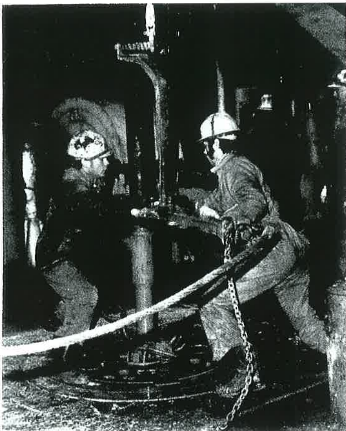
FIGURE 3.4 Applying the tong to make up the drill pipe on the rig floor of British Petroleum's rig, Sea Conquest. Courtesy of British Petroleum.
