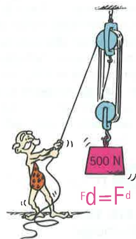
FIGURE 3.32 Applied force \times applied distance = output force \times output distance.
