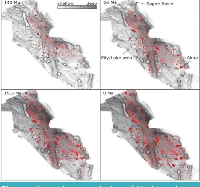
Flow paths and accumulation of Hydrocarbons from coaly source rock over time
