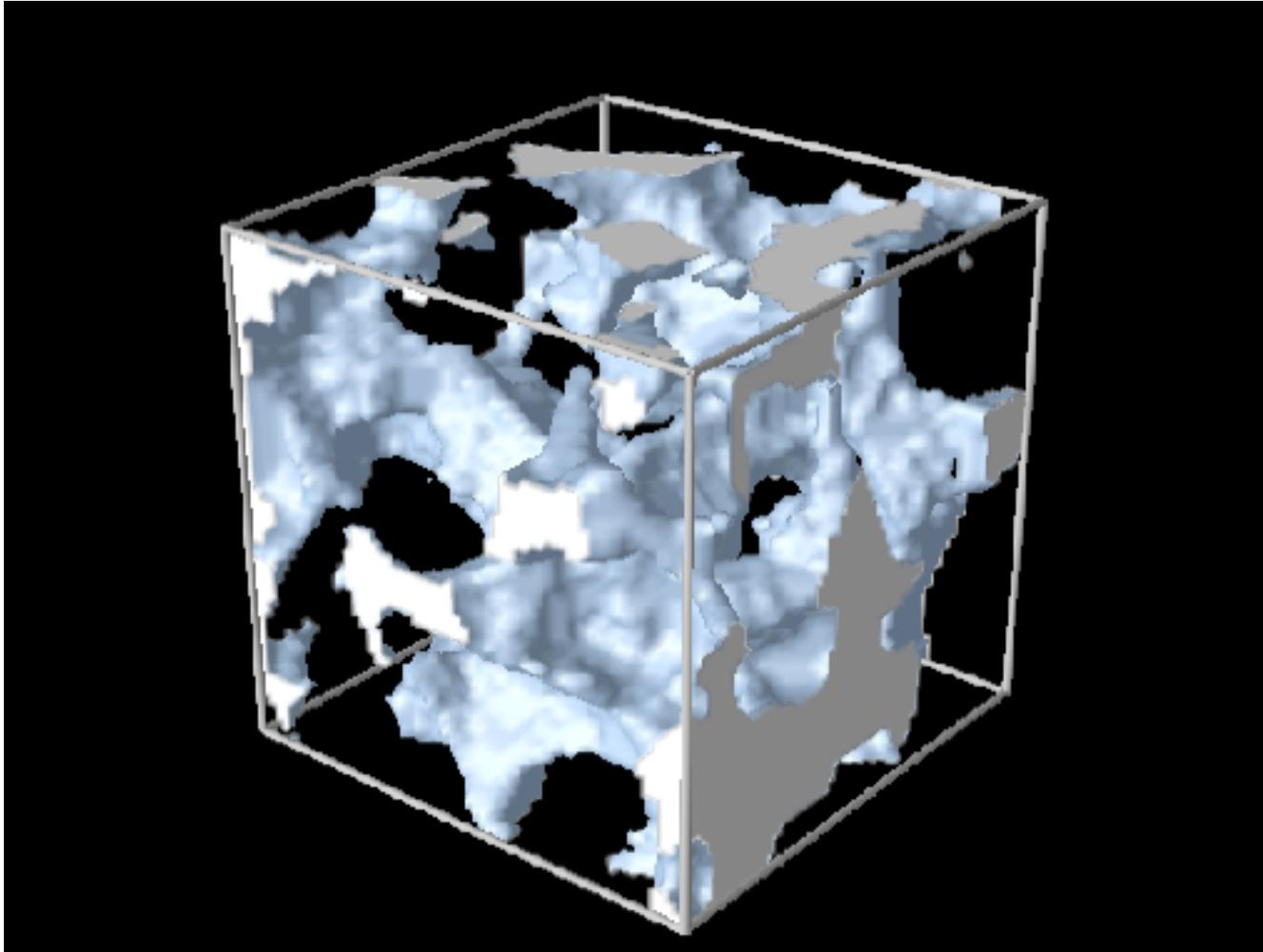
Synchrotron tomography of sandstone.
