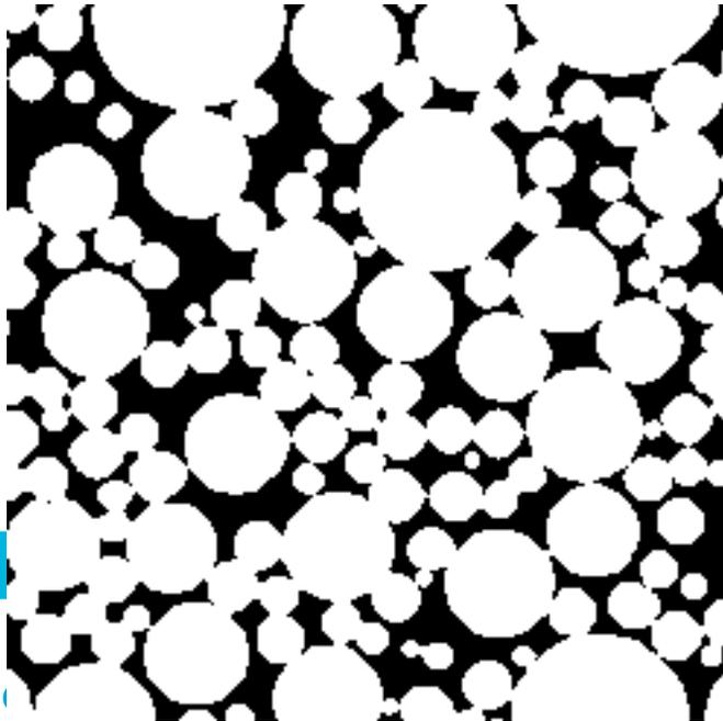
A slice through a granular system such as a sandstone might look like this synthetic image. The grains are white, and the pores black. Try to find a way from the left to the right in the pore space. Is this rock permeable? And what is its porosity?
