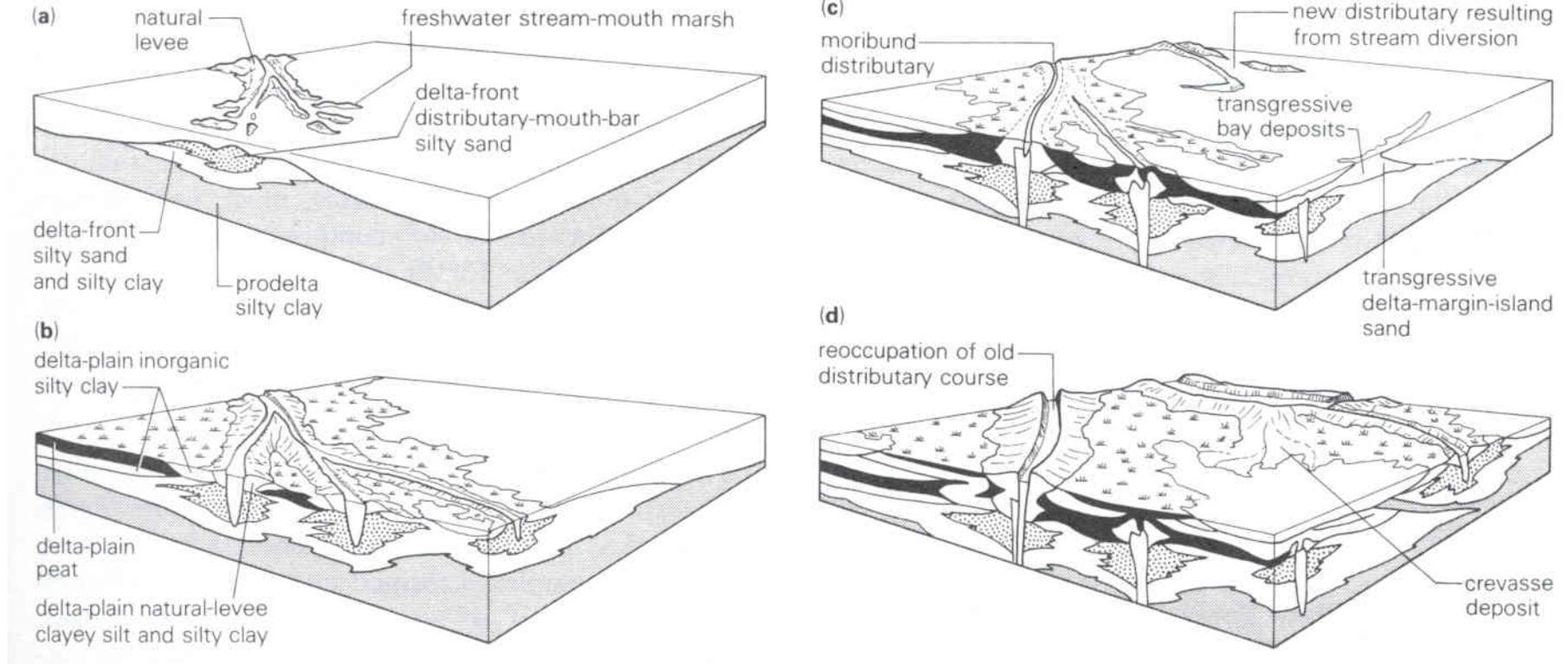
Conceptual depositional models are important in helping to relate well data to a 3-D reservoir model. Shown here are four stages in the formation of a bird-foot delta, such as the Mississippi delta, where rivers dominate sediment distribution.
