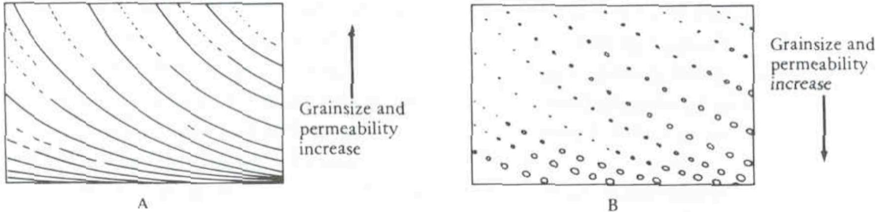
The situation on the left is often found in marine barrier bars, while the one on the right is common in fluvial and marine channel deposits. They are referred to as upward-coarsening and downward-coarsening respectively and lead to anisotropy.
