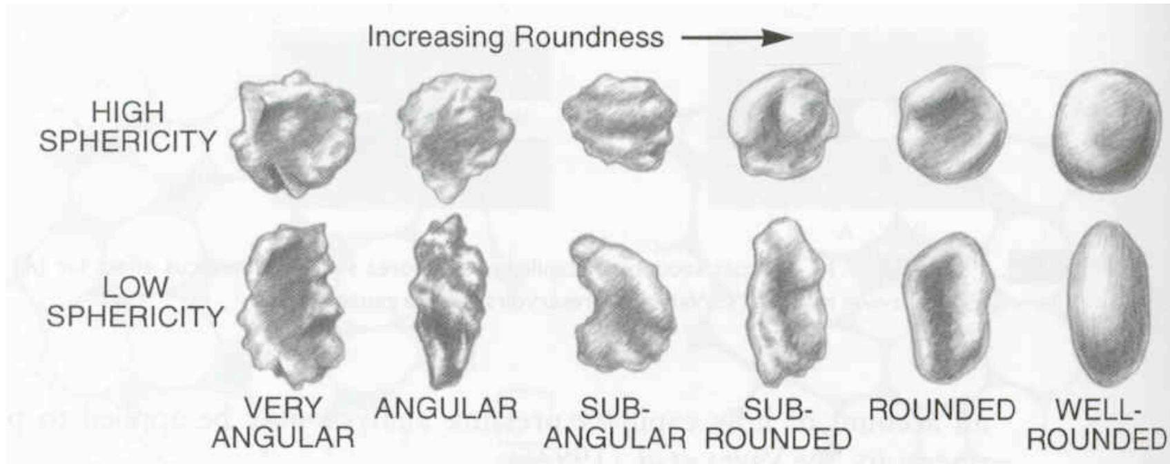
Increased roundness and sphericity lead to higher permeabilities. In what depositional settings do we find the different grains shown here?
