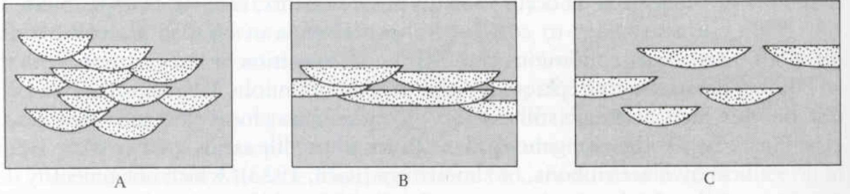
These three sketches show sand bodies with different lateral and horizontal connectivities. A: Vertically stacked (multistorey); B: Laterally stacked; C: Isolated.
