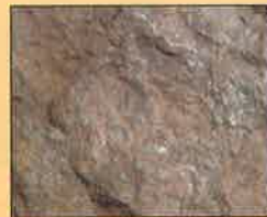
Ironstone: made mostly of iron-bearing mineral crystals like this hematite
